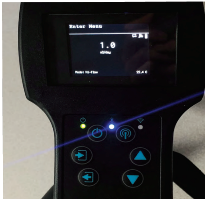
Figure 2.4 Ventbuster® Comms Unit Keypad and Display
