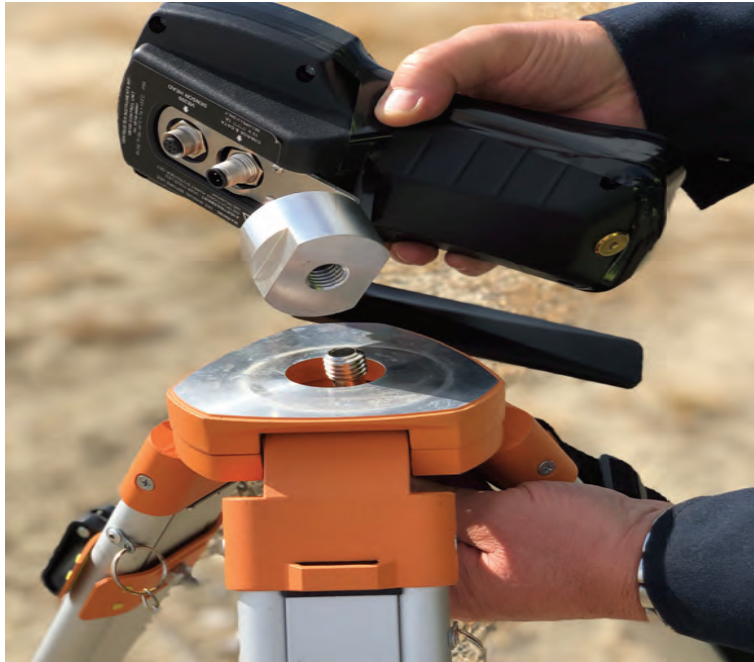
Figure 2.5 Ventbuster® Comms Unit Tripod Mount
